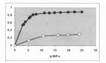
figure 4 Viscosity reduction of liquid Poly-(ethylene glycol) (MW=400), represented by closed circles and expressed as a fraction of the viscosity of the pure polymer, as a function of pressure of carbon dioxide. The open circles represent the composition of the liquid, in mole fraction of carbon dioxide.
